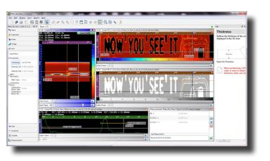
Full recordability of data when using the Prisma is standard, which means that screenshots and all data can be retained and analyzed at a later date using UT Studio. IN using the full data gathering capability - traceability can be achieved; hence repeatability of the inspection and results can be confirmed.
