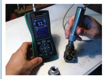
The ultrasonic contact impedance (UCI) probe is used for measuring the hardness of small items, objects with a thin wall, complex form, and to measure the hardness of surface hardened layers.
