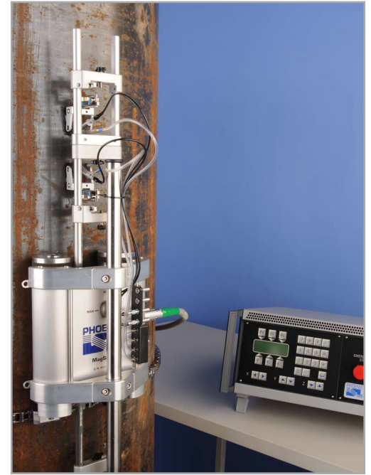
MagScan configured for ToFD inspection
