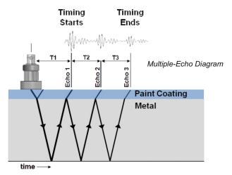
With Multiple-Echo, readings are taken by measuring the time delay between any three consecutive backwall echos. The time of T1 (coating thickness) is ignored. The times of T2 and T3 are equal to the time that it takes to travel through the metal. Only by looking at three echoes can the measurements be automatically verified (where T2 = T3).
