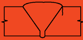
10 Toe Crack in Single Vee MT/PT, UT
