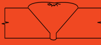
20 Crater Crack (crown stop-start area) MT/PT, UT
