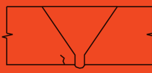
19 Base Metal Crack in Single Vee (bottom HAZ area) MT/PT, UT
