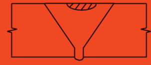
17 Transverse Crack in Single Vee, flush crown MT/PT, UT
