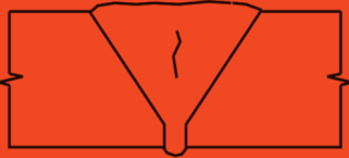
15 Centerline Crack, Single Vee (sub-surface) UT, RT
