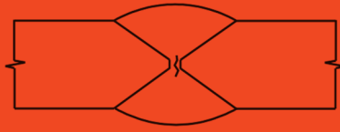
15 Centerline Crack in Single Vee (sub-surface) UT, RT
