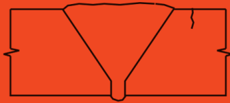
18 Base Metal Crack in Single Vee (top HAZ area) MT/PT, UT
