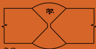
30 Porosity in Double Vee (sub-surface) UT, RT
